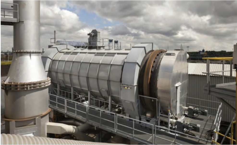
Figure 5.2 The HERA system for recycling asphalt
