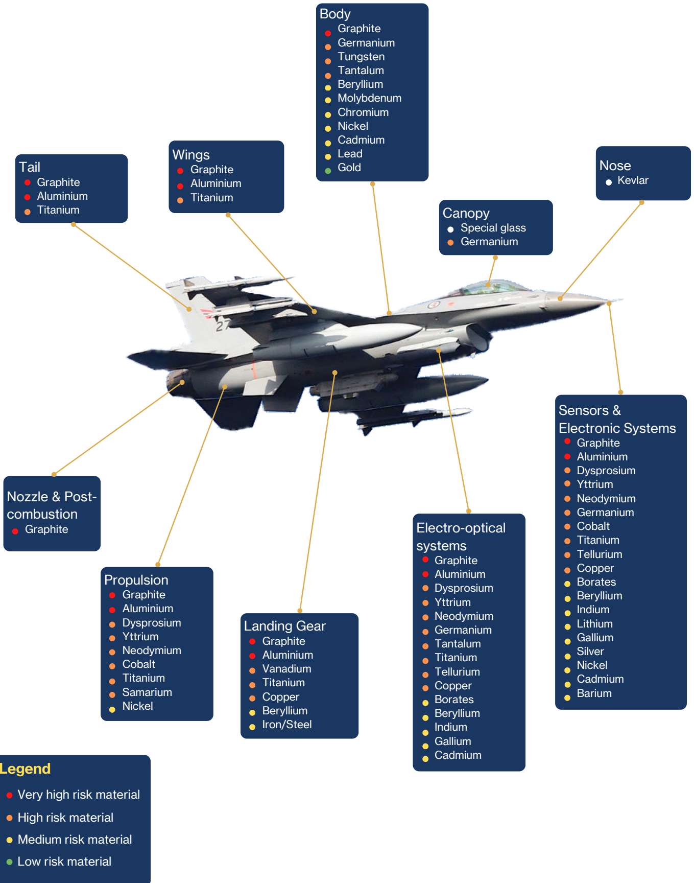
Figure 8. Use of raw materials in a fighter aircraft
