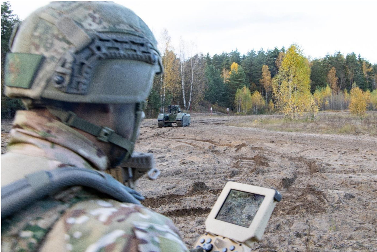
Figure 1. Operator and THeMIS. The operator uses the Remote Controlled Weapon Station which is (digitally) integrated on the platform. Pictured in Lithuania in 2022. Ministry of Defence.
