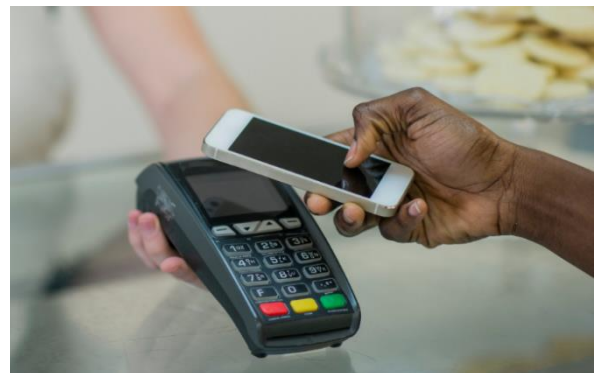
Figure 2. Near-field communication (NFC) technology is used in contactless payment systems.
