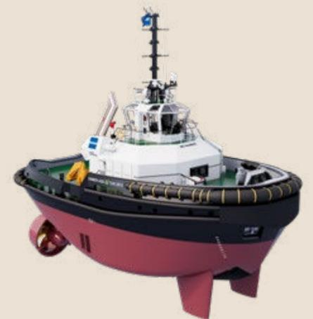
Our concept for an Azimuth Stern Drive 2613 Tug ...but on methanol.
