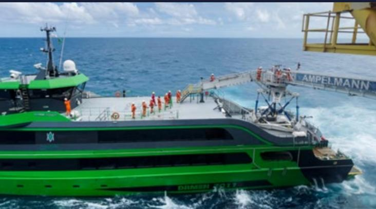
The *Aqua Helix* is the first Damen Fast Crew Supplier (FCS) 7011. The vessel offers a fast, cost-effective and, crucially, comfortable and safe alternative to helicopter transfers offshore for over 120 passengers at a time.
